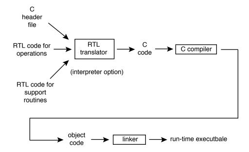
For the interpreter, Icon programs are translated into an intermediate form, which is then interpreted by iconx. iconx's interpreter loop calls the operations and support routines in the run-time system as needed.
