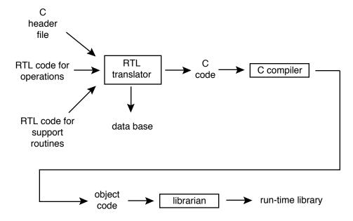
The Icon compiler produces an executable program from Icon source code by translating Icon procedures into C functions, supplying a C main function, and compiling and linking these functions with the library produced using rtt. The compiler makes use of the data base when performing the translation:
