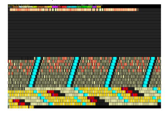
Finally, the display below shows memory after the saved space has been compacted to the beginnings of the regions. The space in the string region is shown as a single string. Since overlapping substrings may be created after strings are allocated, the identification of the ends of strings after garbage collection is somewhat problematical and is not shown.
