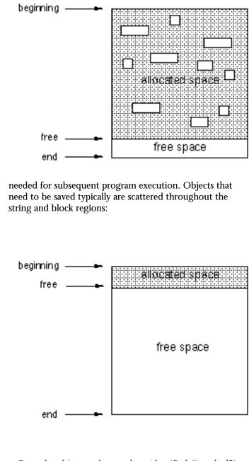
Once the objects to be saved are identified ("marked"), they are relocated toward the beginning of their region, compressing the allocated space and making more free space available so that allocation can proceed:
