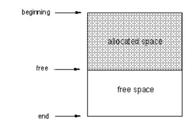
beginning of the region. A "free" pointer is incremented to mark the boundary between *allocated space* and *free space*
