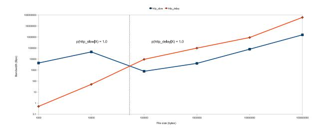
Figure 9: The IFTD-measured bandwidths of two different HTTP implementations for different file sizes. IFTD chooses http\_slow for smaller files since it has a higher average bandwidth than http\_delay for small amounts of data. IFTD chooses http\_delay over http\_slow once the files become big enough that transferring it with http\_delay is faster.
