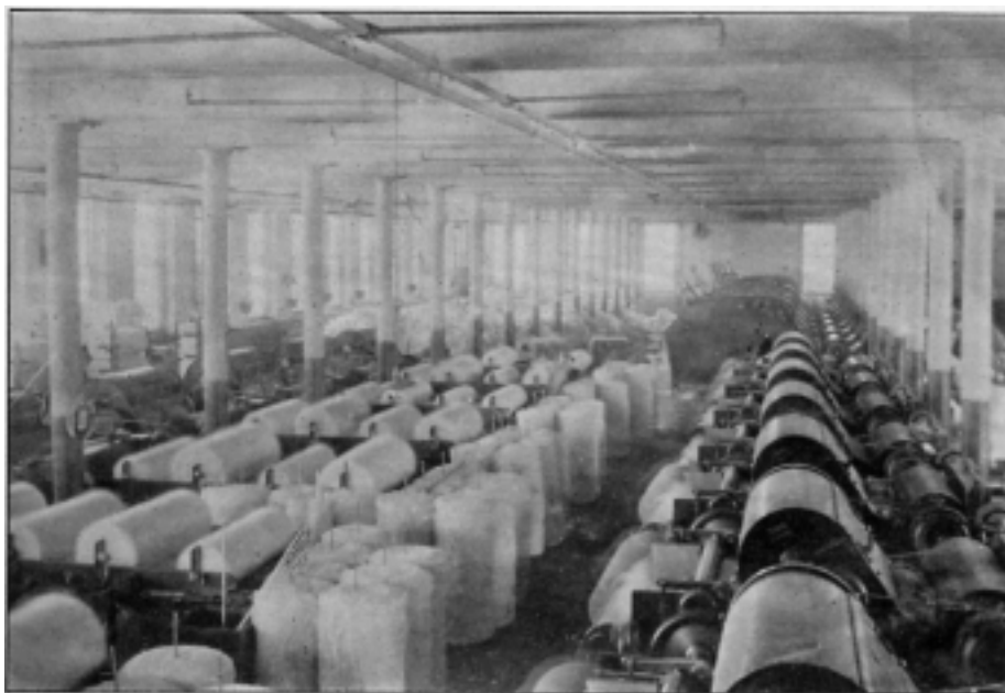
FIG. 10.—A LARGE PICKER ROOM DRIVEN BY DIRECT-CONNECTED MOTORS
