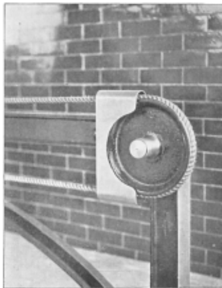
FIG. 17.—END DRAWBAND PULLEY WITH GUARD
