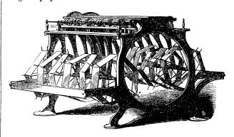
Our drawing represents the winding machine as made by Mr. Frost of Macclesfield, the skeins of raw silk are put on to the swifts which are six-armed reels, with string cross bars to form the fork in which the skein lies. The axles of the swifts lie loosely in centres, and the framing descends no lower than this centre, so that there is very little liability to knocking. The thread is passed through glass guides, arranged on a traversing guide bar, to the bobbins.
