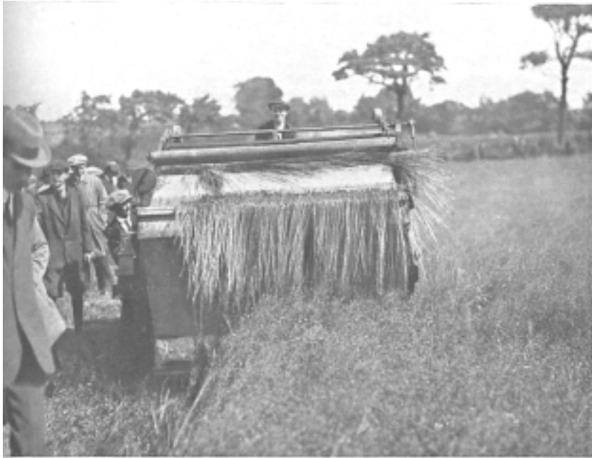
FIG. 1.—The Crawford-Bennett Flax Pulling Machine.
