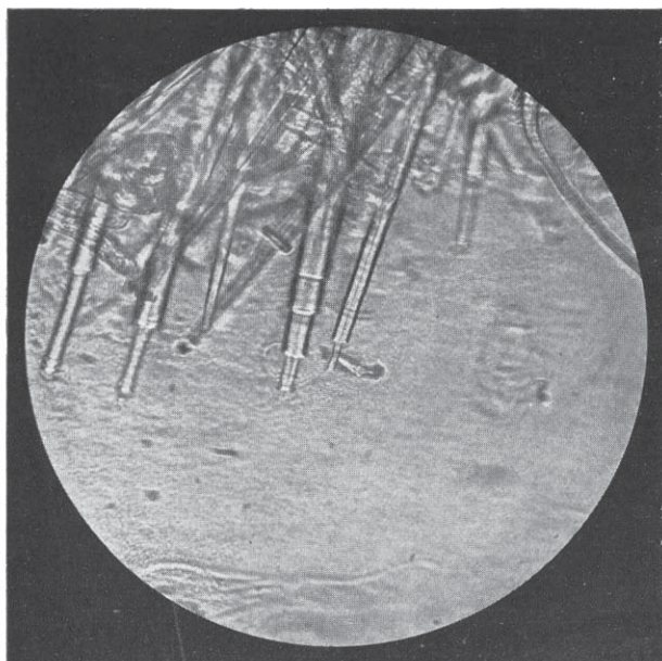
Figure 2 Bamboo Fiber X200 Magnification Setback formation caused by presence of transverse elements.
