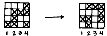
FIGURE 4. TIEUP CHANGE TO INTERCHANGE WARP LAYERS
