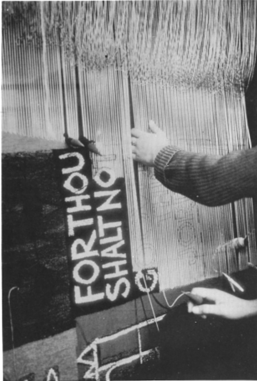
Fig. 7. Using warp threads as a guide for reaching the appropriate leashes for the next row.
