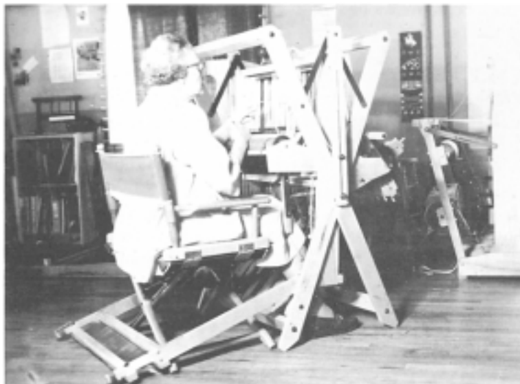
A folded Gilmore loom being threaded by Mrs Martha Ebener, Portland, Oregon
