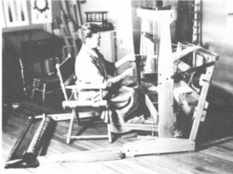
A dismantled Macomber loom being threaded by Helen Bontecou, National City, Calif
