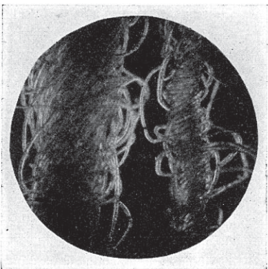
Fig. 7. Faulty twist distribution in woolen yarn. The yarn at left is normal—that at the right has been over-twisted and seriously weakened
