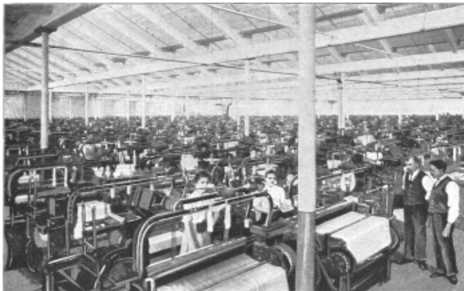
A ROOM FULL OF POWER-LOOMS IN A NEW ENGLAND COTTON-MILL.
