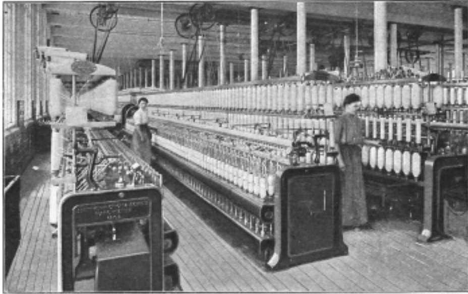
INTERMEDIATE AND ROVING-FRAMES, ON WHICH THE COTTON IS STILL FURTHER TWISTED.
