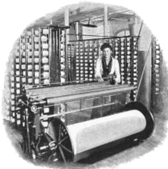
WARPING-FRAME, WHERE THE THREADS ARE ARRANGED FOR THE FIRST OPERATION OF WEAVING.
