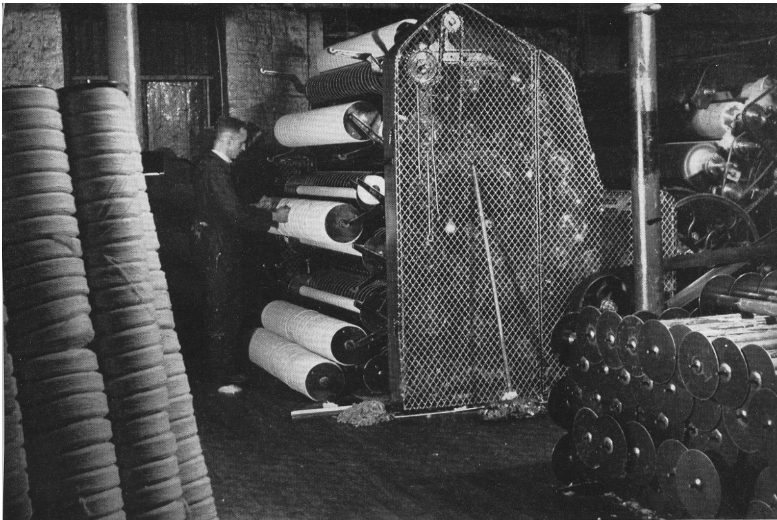
Slivers from the condenser at the end of the carding machine are being wound on to the condenser bobbins. There is no twist in the slivers, and the fibres would part under tension.
