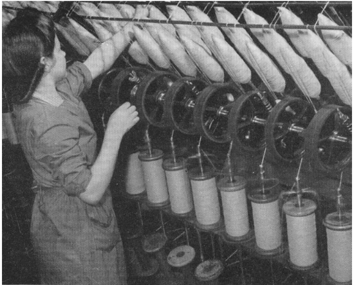
Doubling, an operation which here consists of plying together three ends of spun yarn from three bobbins or cops on to one spindle.
