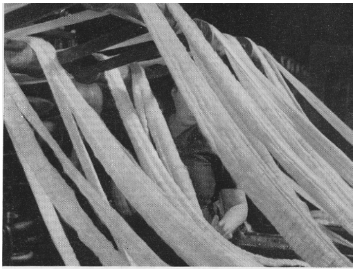
Sets of combed slivers from eight heads or cans are being fed together into each gill box.
