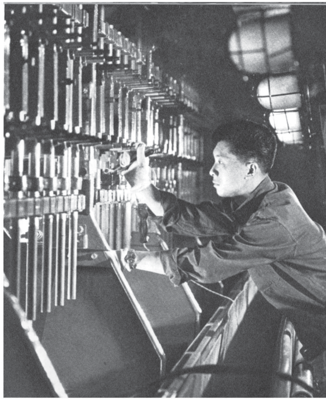
Installing a filament spinning machine, which is now in operation
