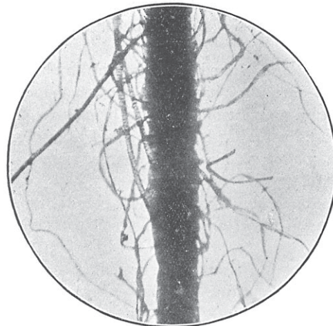
FIG. 9a.—Union yarn. Micrograph of cotton and wool mixture yarn. (a) (b)
