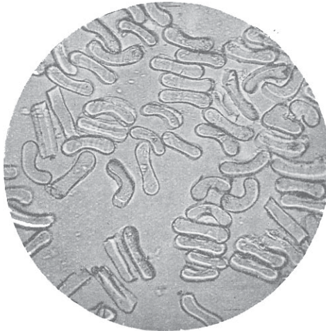
FIG. 44B.—ARTIFICIAL SILK—ACETATE SPECIMEN.
