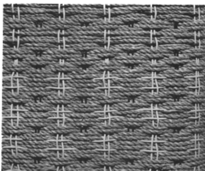
159. Matting sample. Seagrass weft across warp of plastic-covered wire.
