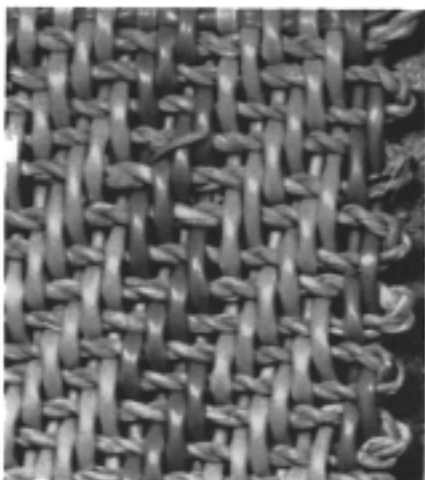
156. Matting sample. Seagrass weft across a warp of plastic tubing, 2/2 twill.
