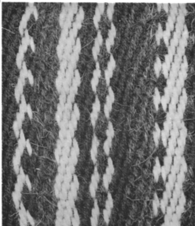
149. Warp-face 2/2 twill, with various colour sequences in the warp.
