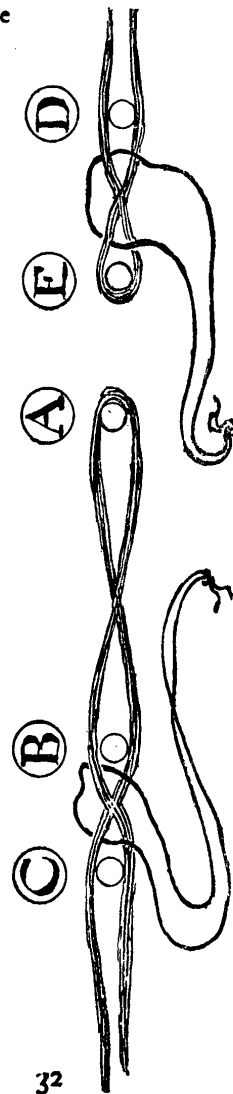
FIG. 15.—Method of securing the Crosses in Warps.
