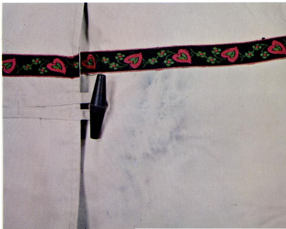
FIGURE 36 The black interlining of this car coat bled to moisture, staining the outer tan cotton fabric.
