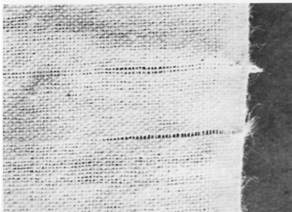
l An attempt to correct a Jerk-In during the weaving of a fabric often leaves a crack in it.
