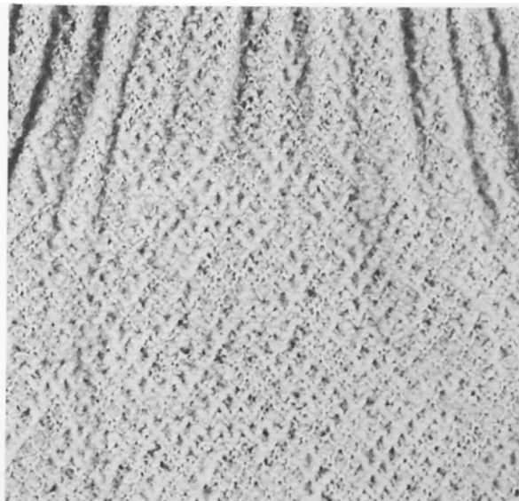
FIGURE 153 Use of water in spotting took the pleats out of this knit fabric. Such novelty pleats, once lost in wear or drycleaning, cannot be reset.
