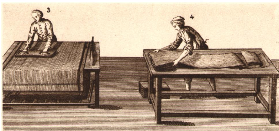
The Woollen Industry at the end of the Eighteenth Century: Disentangling (3) - Folding before pressing (4)
