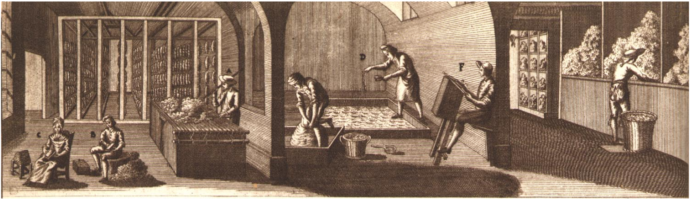
The Woollen Industry at the end of the Eighteenth Century: Beating (A) - Carding (B-C) - Oiling (D) - Opening (E) - Warehouse
