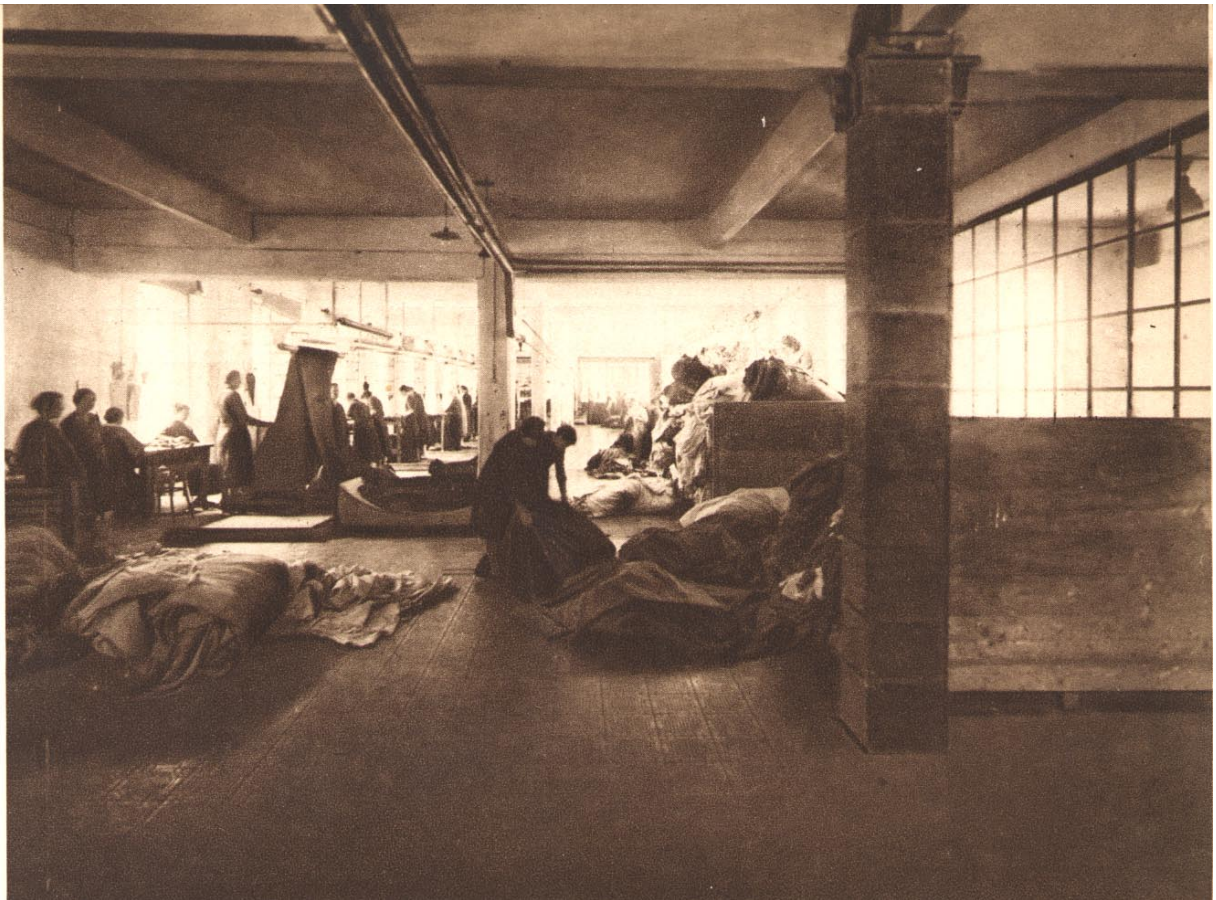
Inspection and Marking of the Pieces
