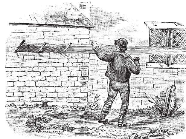
FIG. 150.—PEG WARPING, AN ANCIENT ENGLISH METHOD.
