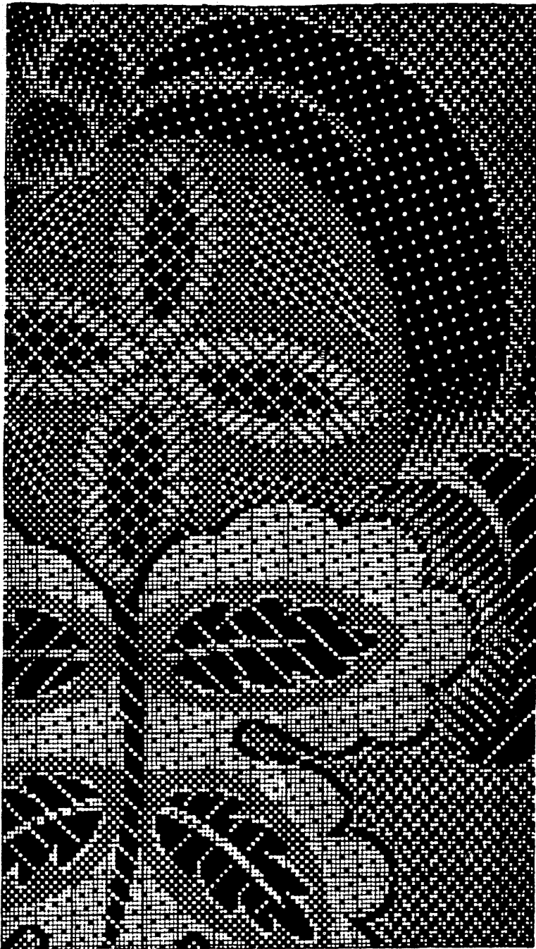
FIG. 540.—Part of an applied design for a brocade fabric with both warp and weft figuring developed in several different weaves to obtain variety of effect as in sketch design, Fig. 539.
