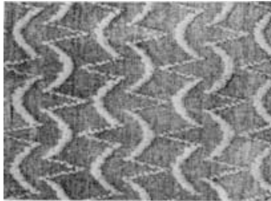
FIG. 519.—Lappet figuring developed by two needle-frames.
