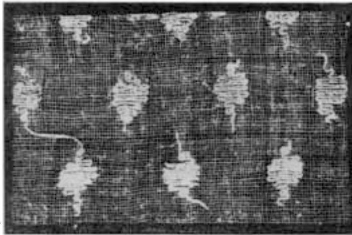
FIG. 517.—Simple spot lappet figuring developed by one needle-frame.
