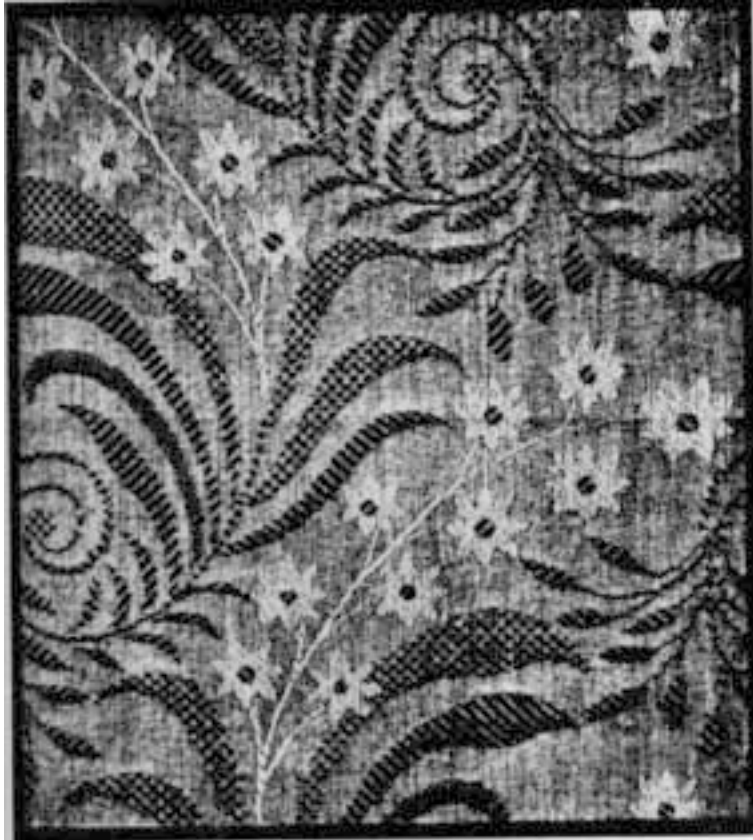
FIG. 538. —Cotton brocade fabric with both warp and weft figuring and a ground weave of plain calico.
