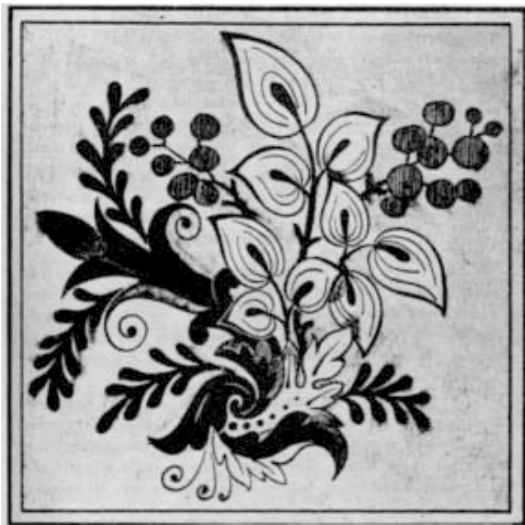
FIG. 543. —Part of a sketch design for a brocade fabric, with both warp and weft figuring, in which extra warp threads, of a different colour, are introduced in certain parts only, to develop the small berries.
