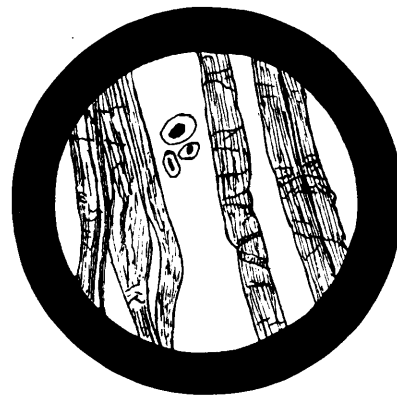
SPECIMENS OF HEMP FIBRES, MAGNIFIED, Showing also Cross Sections.
