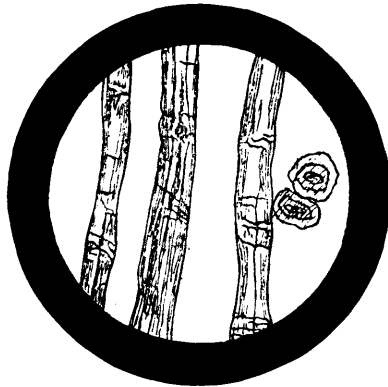
SPECIMENS OF FLAX FIBRES, MAGNIFIED, Showing also Cross Sections.
