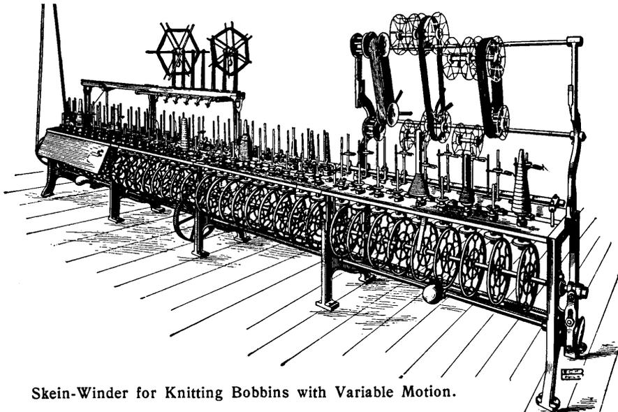
Skein-Winder for Knitting Bobbins with Variable Motion.
