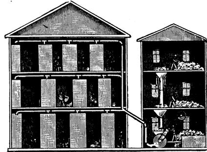
an arrangement of a system of bins, to any one of the latter which may be desired, either in the lower or the upper stories of the mill, or any building, as shown in the accompanying illustration, and the same can be conveyed to any particular place without any possibility of mixing or exchanging stock, as nothing is left in the pipes or against the valves.
