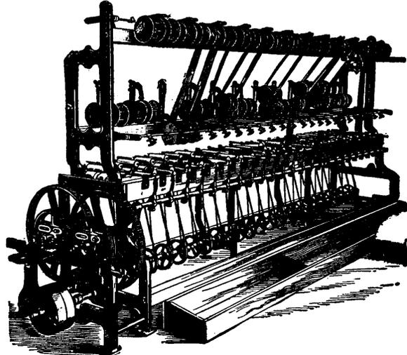
Patent Skein-Winder for Shuttle Bobbins with
