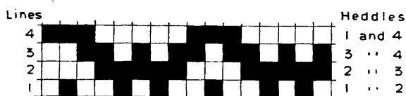
B. Working Drawing of Heddles lifted in Pairs.
