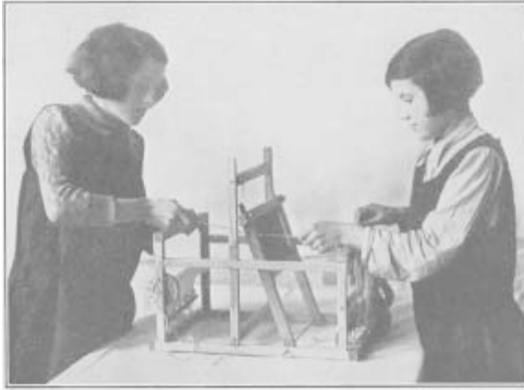
PLATE 34.—ENTERING THREADS THROUGH THE REED READY FOR BEAMING.
