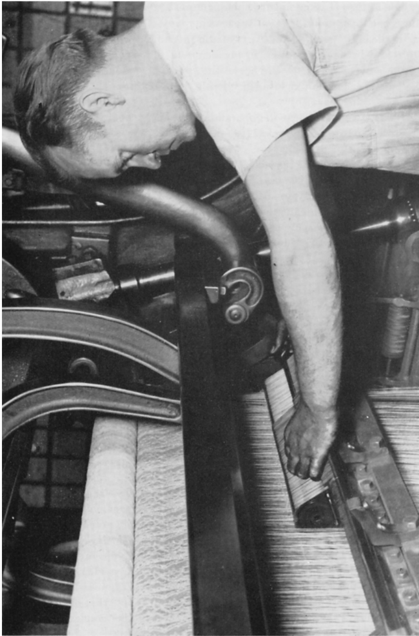
Removing a set of carriages
