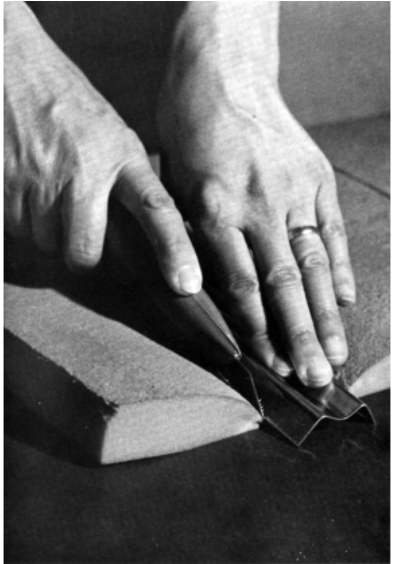
Figure 29 Cutting polyurethane foam with a craft knife and a safety rule
