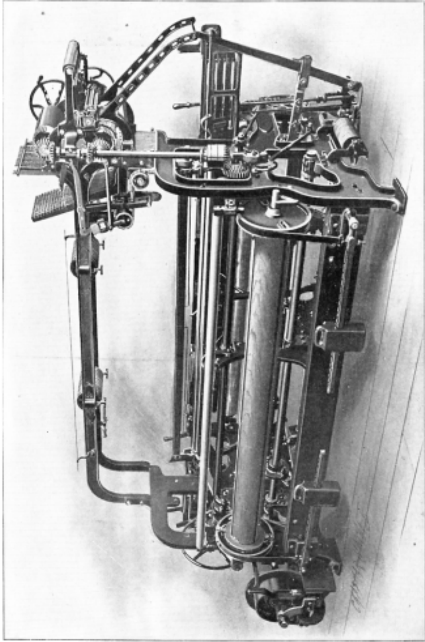
CASSIMERE LOOM WITH 92-INCH REED SPACE Crompton & Knowles Loom Works
