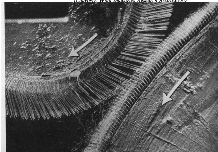
FIG. 7 The action of the Fancy. (Courtesy: Wool Industries Research Association)
