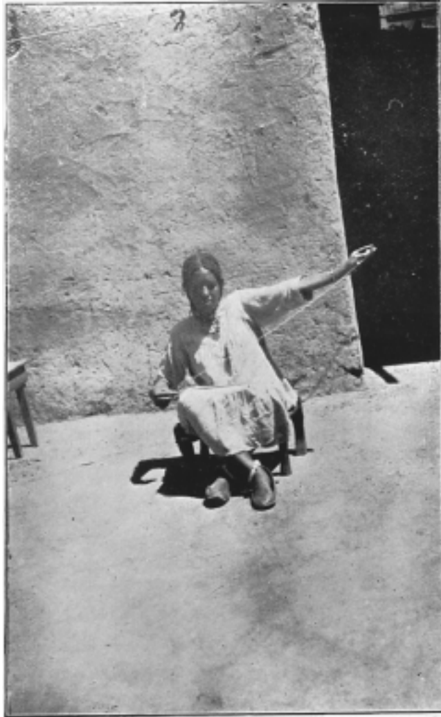
Plate 26.—DRAWING WEFT THREAD WHILE TWIRLING THE SPINDLE IN THE HAND. USUAL POSITION WITH PALM downwards .
