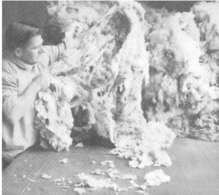
Sorter at work, shaking a lock of matching to clear it of small loose fragments of wool.
