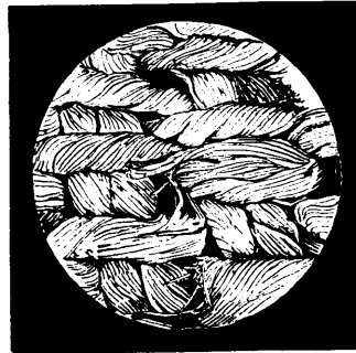
Fig. 27.—Magnified 10 diameters, showing the warp yarn in pairs.
