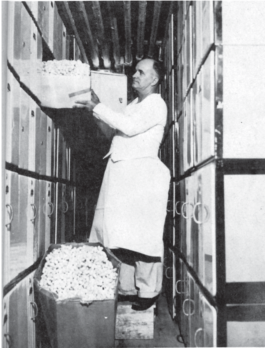
Storing finished cocoons in cold storage plant to stifle chrysalis and prevent moth emerging. These cocoons are to be converted into commercial raw silk.
