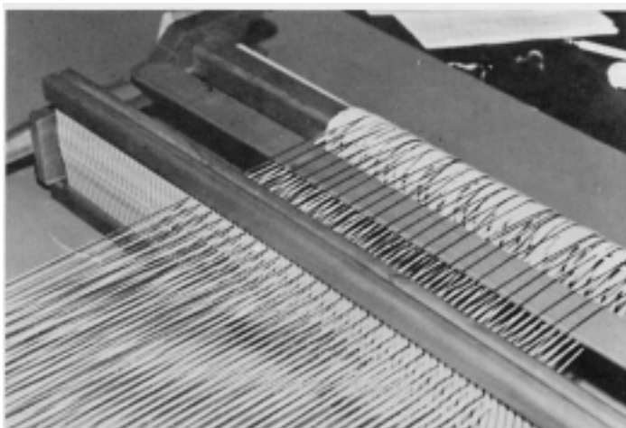
Pickup stick under back heddle slot tiedown threads
