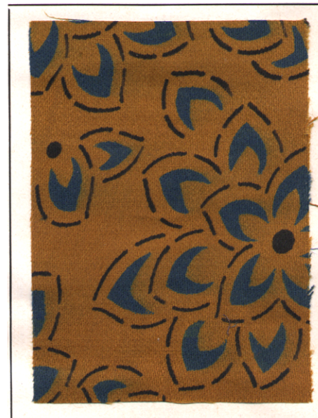
Ground: Ciba Orange G shaded with Ciba Blue 2B Print: Cibanone Blue RSN } Cibanone Blue GCDN } Aniline Black
