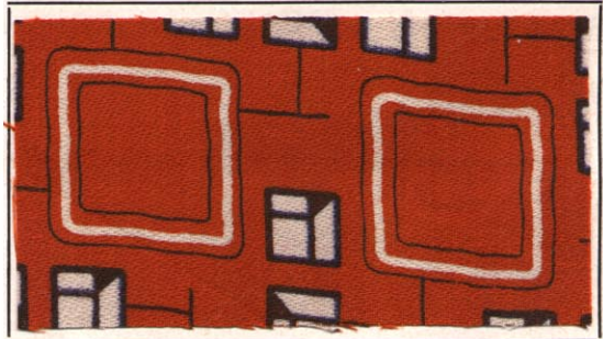
No. 6 Pad: 4% Azol Printing Orange R White: Rongalite C + Citrate Discharge Black: 6% Black for Outlines T
