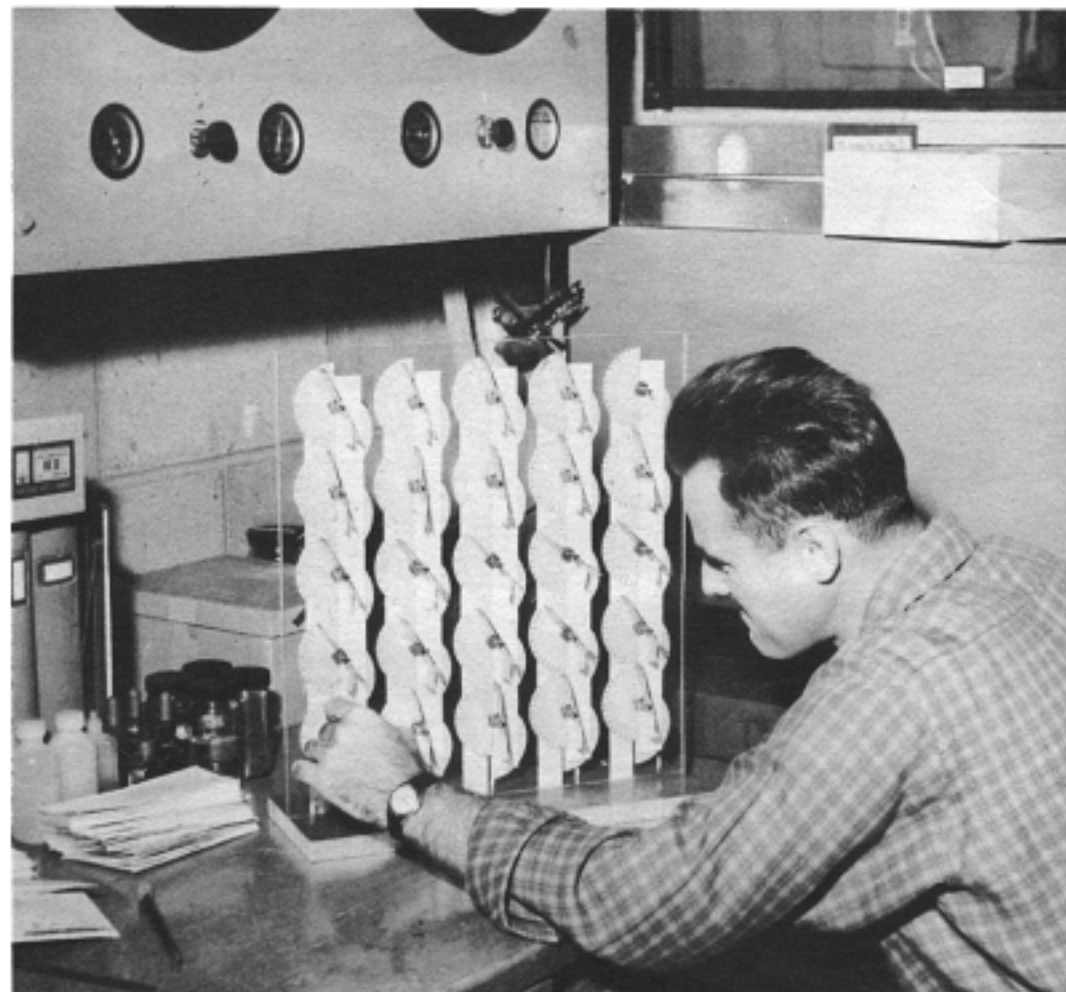
A laboratory technician tests the wrinkle-recovery of sample swatches to evaluate performance
