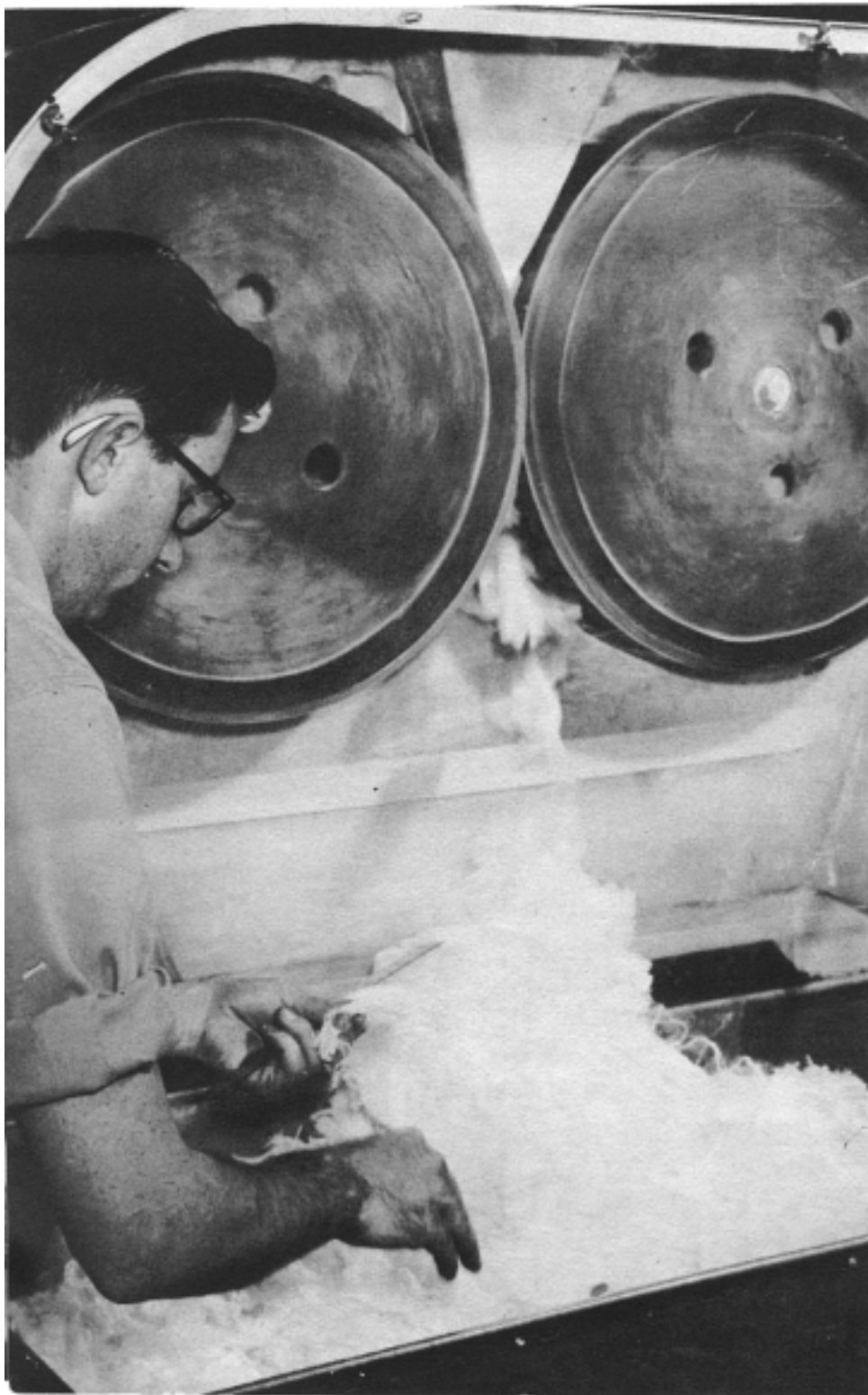
Cutting Zefran into staple fiber is one of the functions performed in the Williamsburg plant
