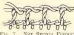
FIG. 7. NET STITCH FINISHED AT TOP WITH RUNNING STITCHES TAKEN IN EVERY LOOP
