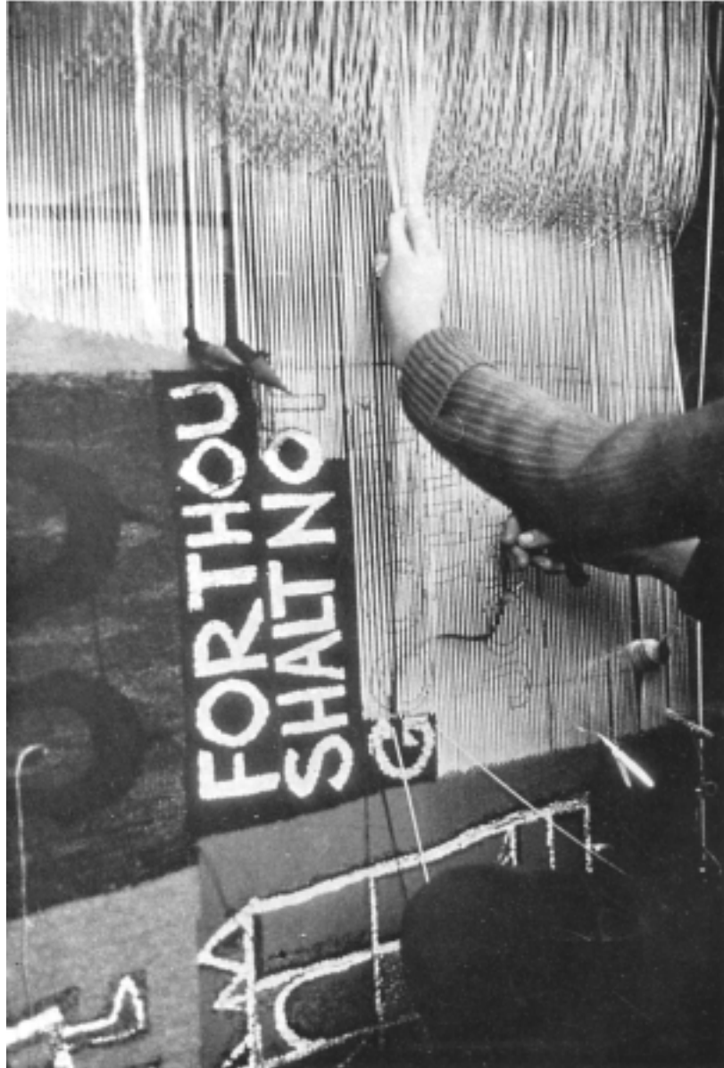
Fig. 8. Bobbin has just been passed from left to right.
