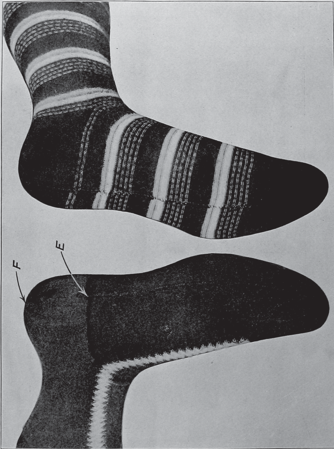
UPPER VIEW: HILSCHER'S WEDGE HEEL FOOT (inner side out) LOWER VIEW: FRENCH FOOT (inner side out)
