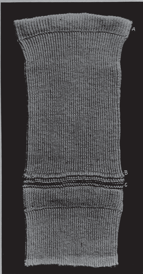
A—Double French Welt. B—Slack Course for Looping on Topping. C—Cast off Course for Separation or Cutting.
