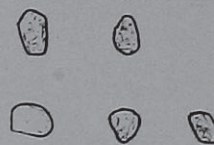
FIG. 3. SECTIONS OF BRINS OF ANAPHESILK, 230 TIMES ENLARGED.
