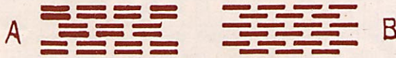
FIG. 9. ARRANGEMENT OF WEFT SKIPS WHEN SUMMER AND WINTER IS TREADLED "IN PAIRS." A: AND "ONE AND ONE." B.
