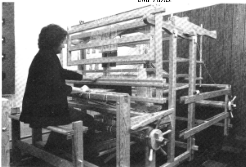
4. View of the Glimåkra damask draw loom showing some of the pattern shafts pulled up with a draw cord
