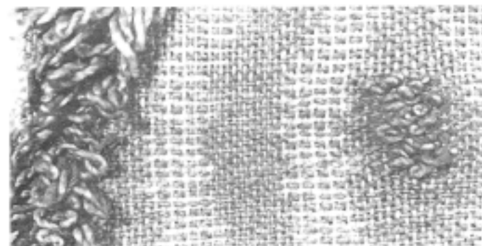
7. Shifting weft. A looped texture takes up the extra yarn and forms a smooth selvedge.
