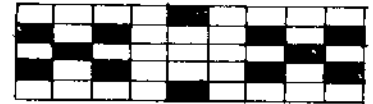
Figure 10.—Design of spots. One spot covers several warp ends depending on the size of the spot.
