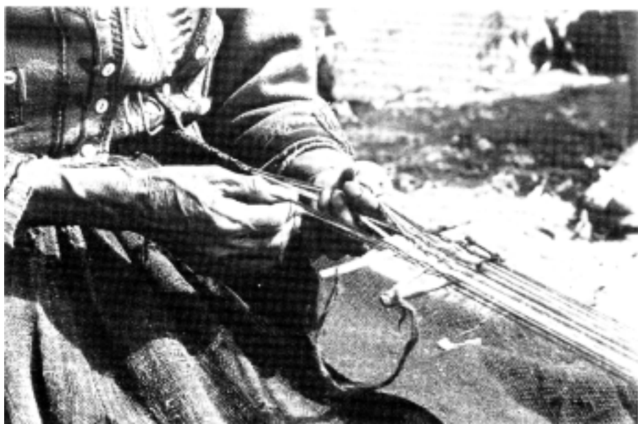
Photo 4. Chinchero: To make a "Tube 5" edging all around a large manta, Benita Gutierrez needs long warps (15' to 20'). She keeps her yarns in order with a tanka , and also uses a holding stick for reserving sheds. Her weft is on a needle, so the edge is attached as it is woven.
